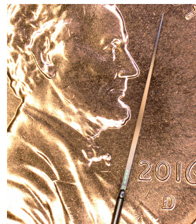
Left: 16- and 32- channel Vector Arrays Below: 64-channel Vector Array on a US penny
