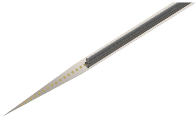
Illustration showing flat optical fiber mounted on an electrode array shank.
